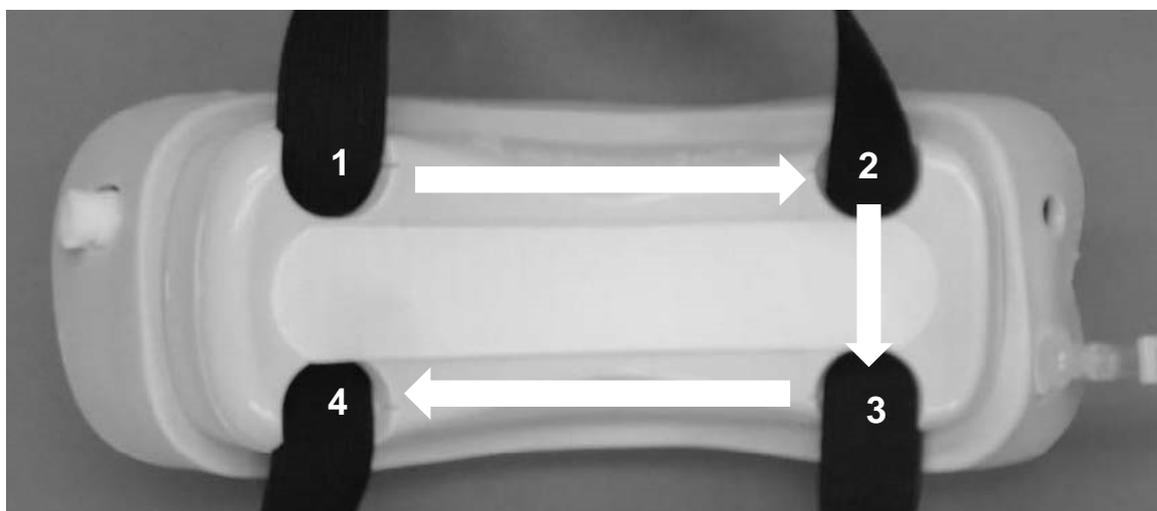
Place the back panel on to the simulator unit and press them firmly before screwing. Fasten the screws following the order shown in the previous page.
