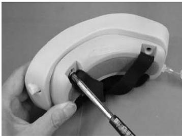
The first screw is to be fastened only lightly at the beginning.
