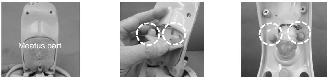
2) Put the two projections at the backside of the skin into the openings in the internal panel to anchor the skin in place.
