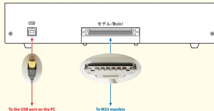
Shown above is the ports on the side of the USB box. Take note the direction of M55 manikin connector.
