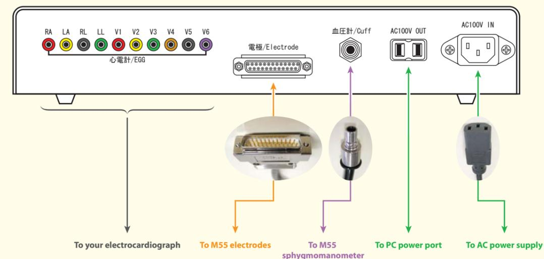
Shown above is the ports on the back of the USB box. Take note the direction of M55 electrodes connector. Your electrocardiographic monitor can be connected by putting the electrodes to each corresponding ECG port.
