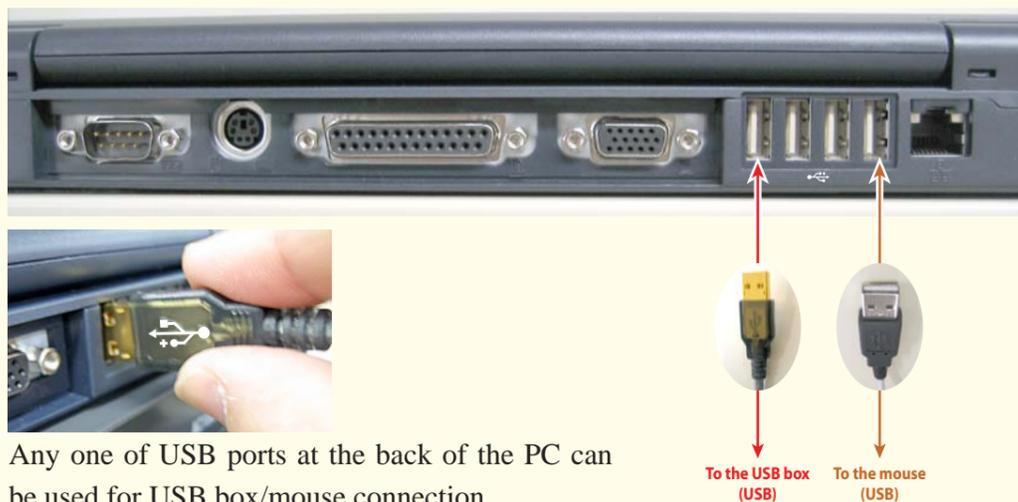
Any one of USB ports at the back of the PC can be used for USB box/mouse connection.
