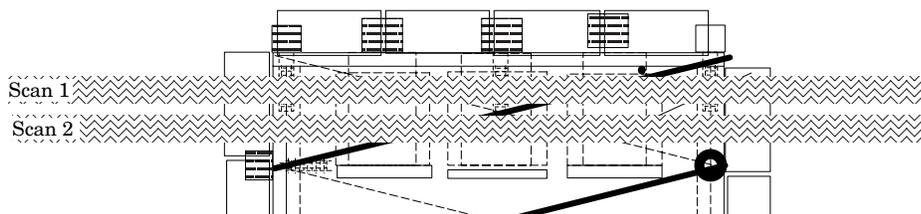
The ramps can be used to test the indexing between slices within a multislice sequence. Set a multislice sequence with an inter scan gap of 0. The sequence should be positioned so the end of the first slice will be even with the center of a test plane. Measure from the center of the first ramp to the center of the second ramp and multiply it by .25 (the 14° scaling factor) to determine the scan index between scans.
