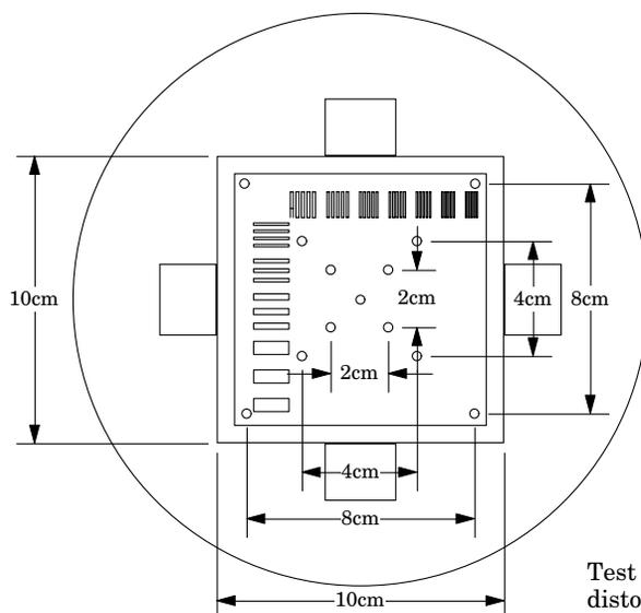
Test cube plane 3, geometric distortion (spatial linearity)
