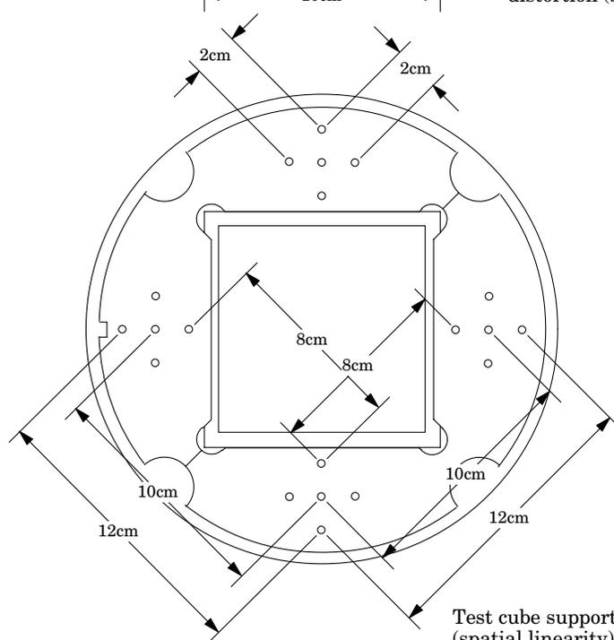
Test cube support disk, geometric distortion (spatial linearity)
