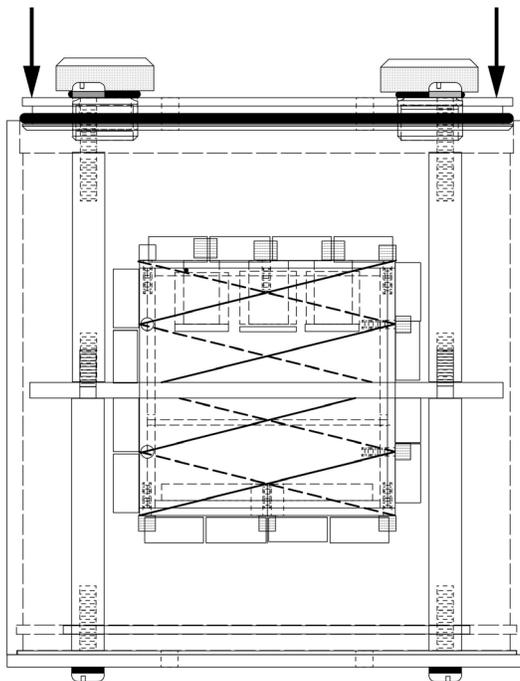
To install the test cube and support disk, the two pieces of the support disk need to be oriented so the wide flanges correspond to the notches in the test cube. Then attach the retaining disks. The cube and disk assembly should then be lowered onto the support posts in the phantom.
