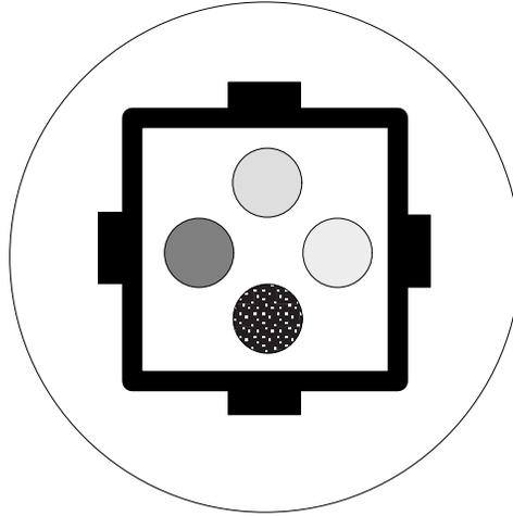
Four sensitometric target vials are found in the top scan plane of the Magphan® test cube. These targets can be filled with your choice of MRI test solutions or gels. For example, four solutions with known systematical varied concentrations can be used. To fill the vials remove the screw plugs on top of the test cube using the hex wrench provided. Do not over tighten the screws after filling the vials.
